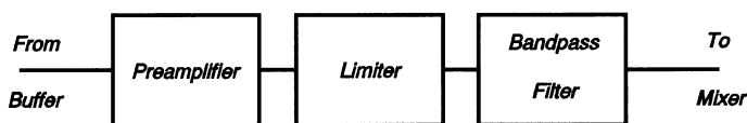
Figure 4.6. A block diagram showing the details of the limiter/filter shown in Figure 4.5.
